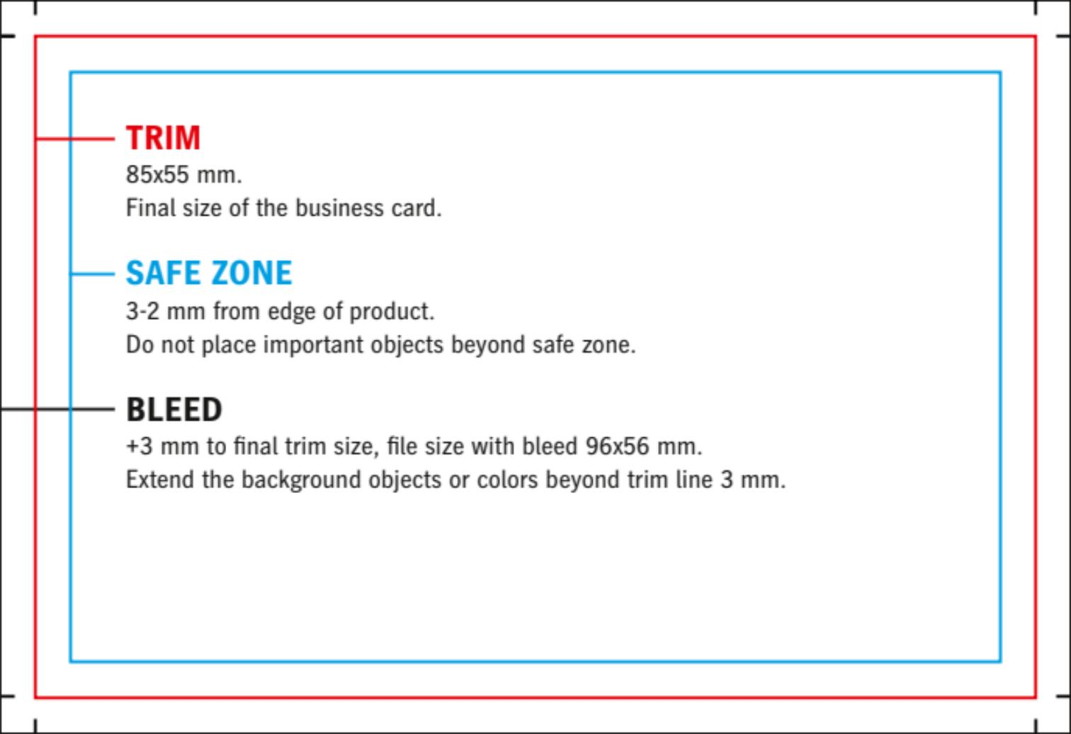
The diagram shows a business card layout with three distinct boundaries. An outer red line represents the final trim size. An inner blue line represents the safe zone. A black line, located 3 mm from the blue line, represents the bleed area. Lines connect these boundaries to their respective text descriptions on the left side of the page.
